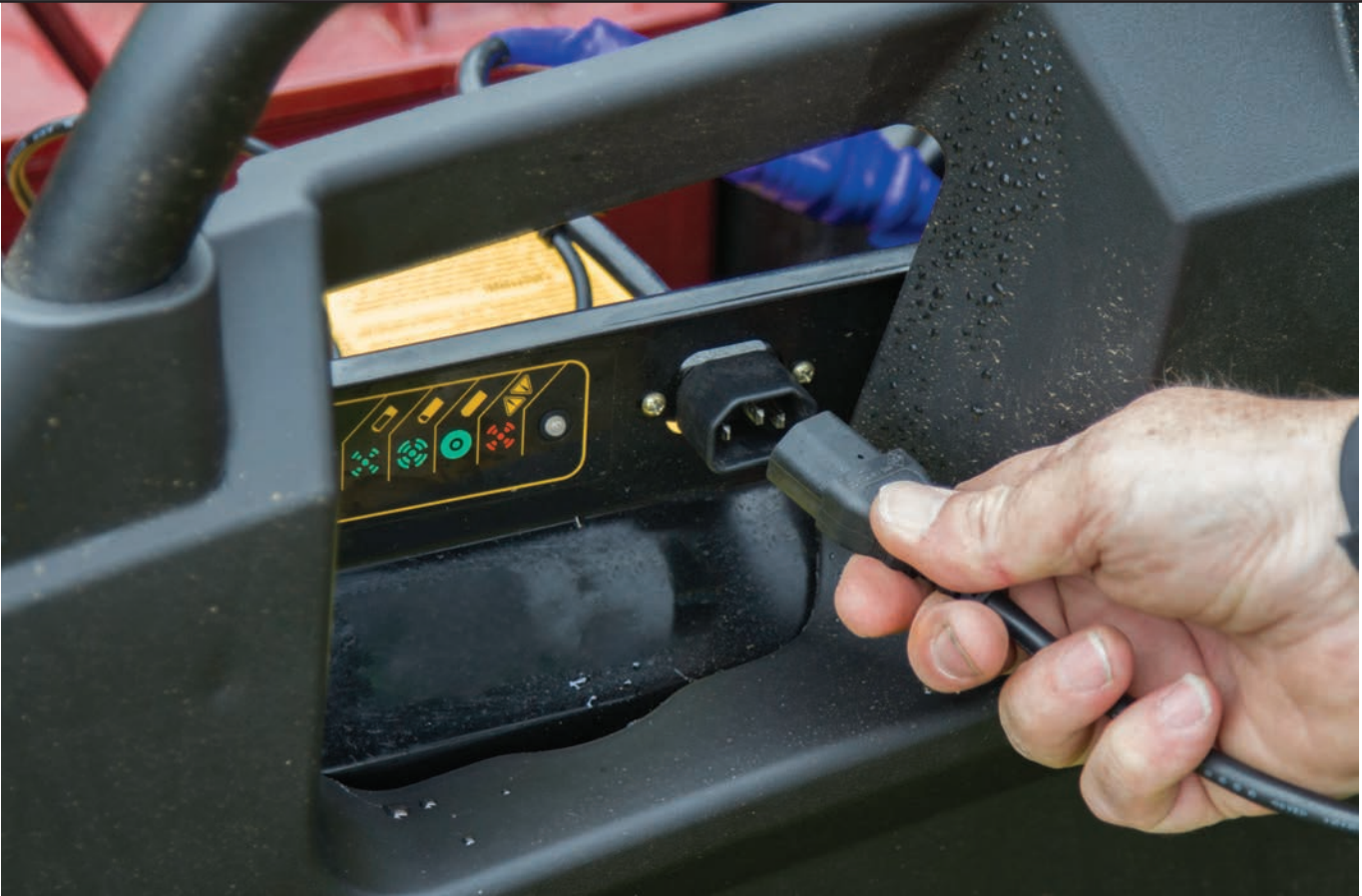
The integral charger runs from a standard 13 amp single phase plug in cable. The charger is designed to either provide a quick top-up or be left hooked to the mains for an extended period
